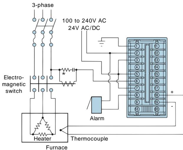
\* Surge absorber: To prevent the unit from harmful effects of unexpected level noise, it is recommended that a surge absorber be installed between the electromagnetic switch coils.
