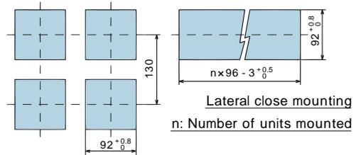
⚠ Caution: When Lateral close mounting is applied, Dust-proof and Drip-proof specification is not fulfilled.
